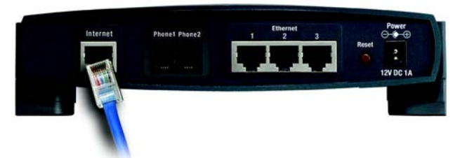
Figure 4-4: Connect the Cable/DSL Modem
