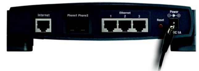
Figure 4-5: Connect the Power
