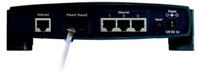
Figure 4-3: Connect a Telephone
